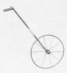
This model measures 5 feet in circumference with 10 spokes placed 6 inches apart so that one can record measurements in both feet and inches. This wheel is especially adapted for overland measurement. The counter registers once for each revolution of the wheel.
